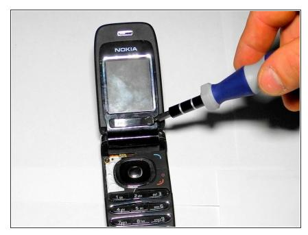
Using a 2.0 flathead screwdriver, pry open and remove the black, plastic strip (beneath the screen) to reveal the 2 screws holding the screen in place.
