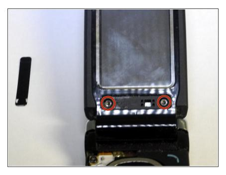
Remove the two T6 Torx screws from the base of the display.
