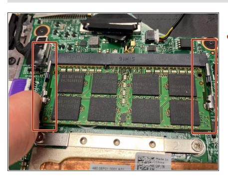
Release the RAM by unhinging the connecting bars outward.
