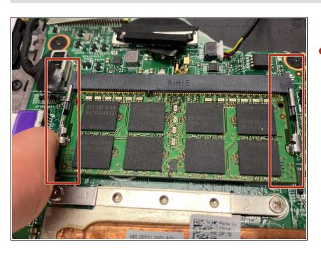
Release the RAM by unhinging the connecting bars outward.
