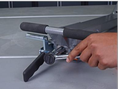
• Use a socket wrench with a deep 9/16" socket to remove the retaining nut and star washer from the control switch toggle.
