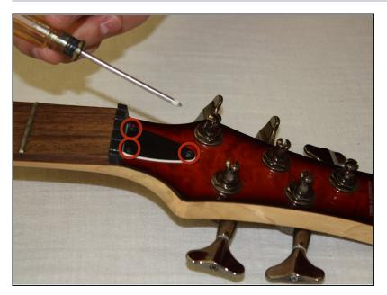
Locate the screws covering the truss rod.
