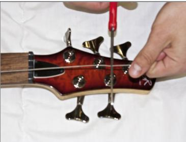
• On a taut string, measure one inch past the nut before using a pair of wire cutters to cut the string.
