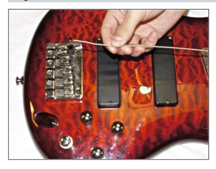
Thread the largest new string through the bridge hole farthest from the knobs. Hold it firmly in place.
