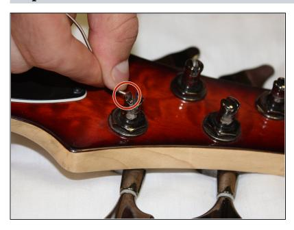
Take the end of the string and insert it into the hole in the middle of the string tree.
