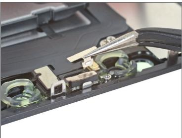
Use tweezers to slide the small bracket straight up and off of the ambient light sensor.
