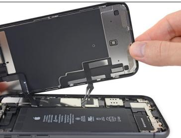
To access the screws in the following step, tilt the display by slightly lifting its lower edge.
