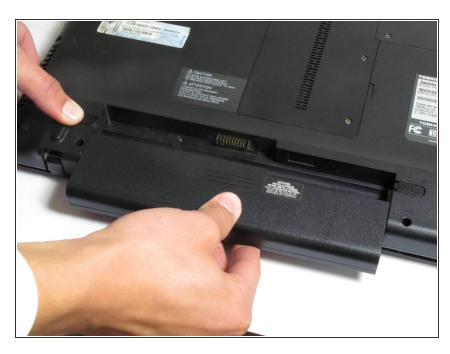
While holding the lock in place, slide the battery out towards you.
