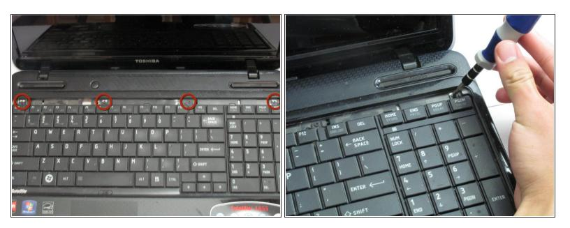
Unscrew the four 3.7 mm screws at the top of the keyboard using a #1 Phillips screwdriver.
