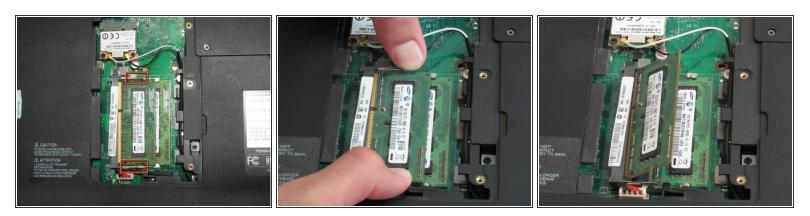
Push the two tabs outwards, away from the RAM. The RAM should spring up.
