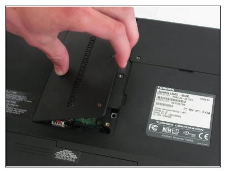
Remove the cover, firmly lifting from the indent. It is recommended that you leave the screws in the panel.
