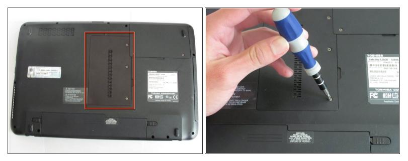
Unscrew the three 4.6 mm screws holding the panel using a #1 size Phillips head screwdriver. The panel is centered on the bottom of the laptop.
