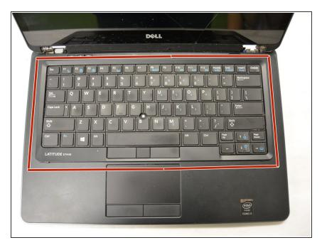
Remove keyboard bezel by using the opening tool to gently pry open the sides.
