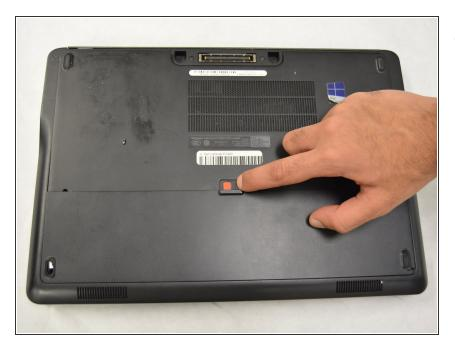
Slide the latch and remove the battery.
