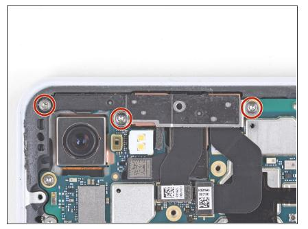
Remove the three 3 mm long T3 screws securing the front camera bracket.
