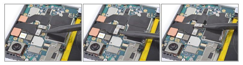
Use the point of a spudger to carefully pry up and disconnect the cameras from their motherboard sockets.
