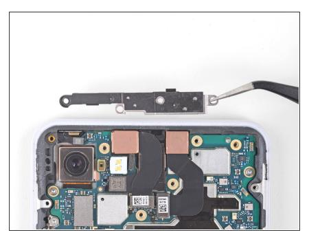
• Remove the front camera bracket.
