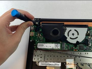
• Remove the three 3.38 mm screws from the left fan (this fan should be black).
