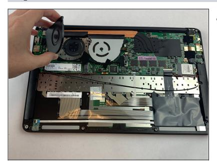
• Carefully lift and remove the left fan.
