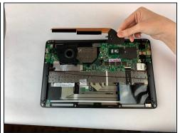
• Once the screws are removed, the piece can be gently lifted from the back of the device.
