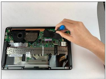
• Remove the four 3.38 mm screws around the black square using a Phillips #00 screwdriver.
