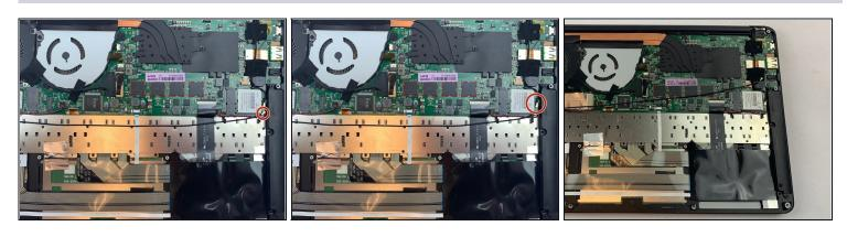
• Carefully remove the auxiliary and main wire from the Killer 1535 wireless card.
