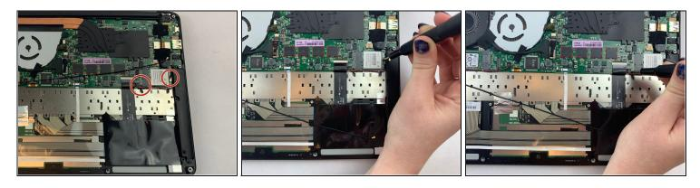
• Use a Phillips #00 screwdriver to remove the two 2.61 mm screw holding the card in place.
