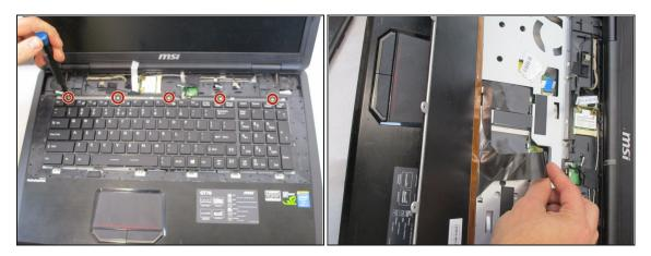
• Using a Phillips #0 screwdriver, remove the five 3 mm screws at the top of the keyboard.
