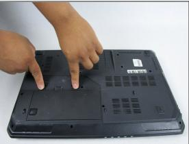
Release the safety latches that hold the battery in place. The left latch will stay moved up, while the right side is spring activated and will have to be held.
