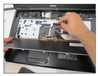
Flip the keyboard back and disconnect the keyboard cable.
