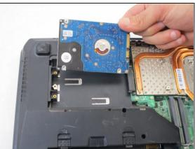
• Slide the hard drive to the left, removing it from its bay.
