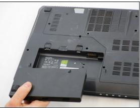
• While holding up the left latch, use a Jimmy and slide the old battery out of its compartment.
