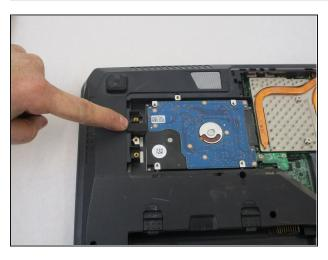
• Remove the rubber spacer holding the hard drive secure.
