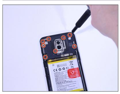
Remove eight 3mm Phillips #00 screws that connect the midframe to the phone.
