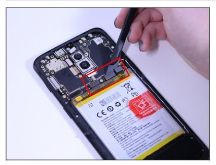
Using a spudger, disconnect the charging port flex connector, the main flex connector, and the screen flex connector at the bottom of the camera.
