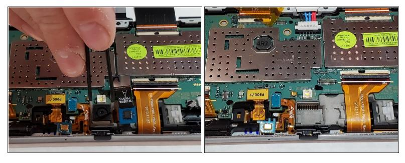
Use tweezers to carefully remove the camera.
