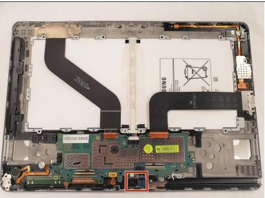
Remove the back cover of tablet with the blue plastic opening tool.
