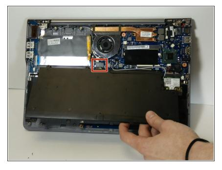
Pull the battery connector towards the battery to disconnect it.
