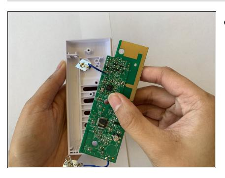
Remove the circuit board
