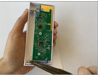
Remove the positive and negative battery contacts using pliers
