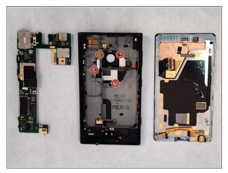
Using a T4 screwdriver, unscrew four 4.60 mm screws to disconnect the rear camera casing from the rest of the device.
