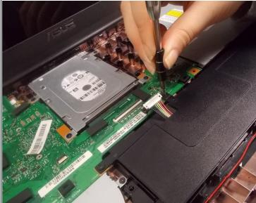
Use Phillips #0 screwdriver (PH0 bit) to remove the four 6.0 mm screws attaching the battery to the laptop.
