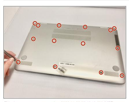
Remove the fourteen 7mm screws using the Phillips #0 screwdriver from the bottom of the laptop.
