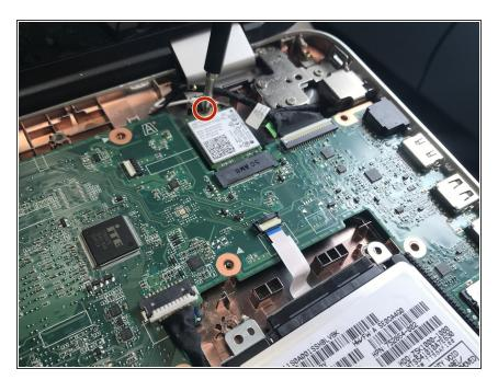
Remove one 3mm screw with the Phillips #00 screwdriver.
