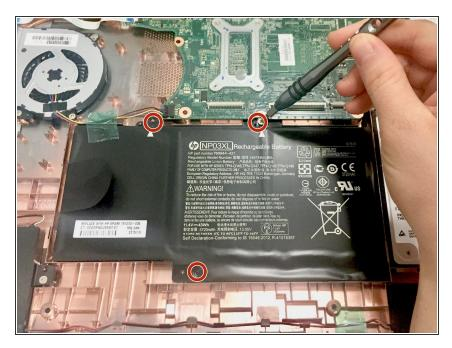
Remove the three 4mm screws using the Phillips #0 screwdriver.
