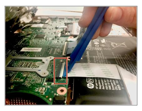
Remove the thick white ribbon cable covering the battery using the plastic opening tool by prying up the latches attaching each end.
