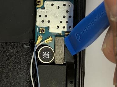
Use a plastic opening tool to undo the connector and the two wires on the motherboard.
