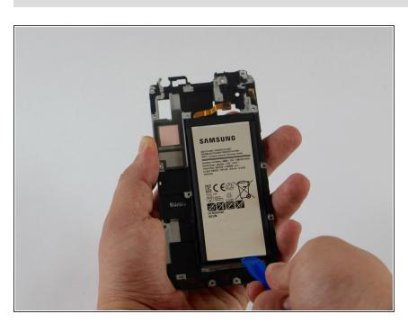
Insert a plastic opening tool on the side of the frame and pull out the battery.
