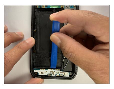
Insert a plastic opening tool under the USB board and remove the USB board from the rear case.
