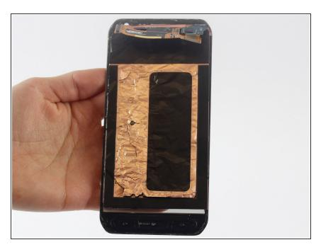
Remove the display assembly (LCD and Digitizer).
