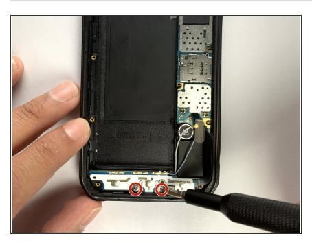
Use the Phillips #000 screwdriver to remove the two 4mm screws from the USB board.
