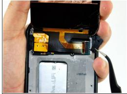
Once the glass is off, you will see a small clip covering the screen connection to the motherboard at the top of the phone. Use tweezers to grab the clip by the crease on its side and pull it out.
