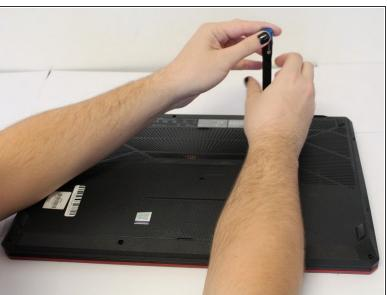
Remove the eleven Phillips #0 screws that secure the back cover.
