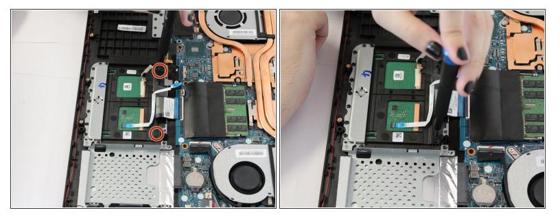
• Use a Phillips #00 screwdriver to remove the two screws holding the track pad in place.
