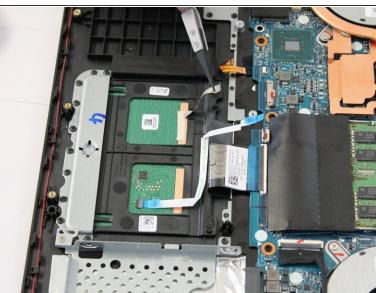
Take the ground wire ribbon and pry it off of the motherboard housing with tweezers.
