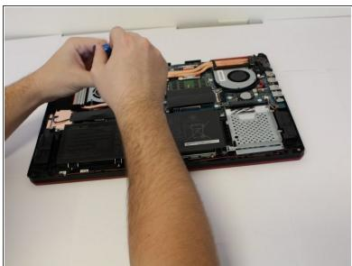
Remove the three Phillips #00 screws from the battery housing.
