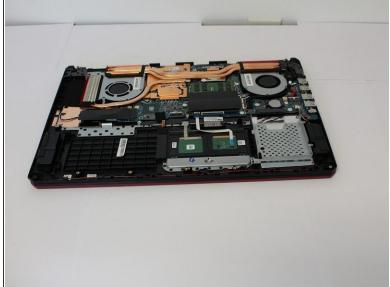
Disconnect the wire from the motherboard, and lift the battery from its housing.
