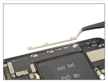
• Remove the flex cable bracket.
