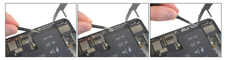
• Peel up the two remaining battery adhesive pull-tabs to un-stick them from the right edge of the battery.
