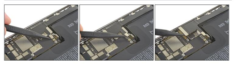
• Pry up to disconnect both of the Lightning flex cable connectors from the Logic board.
