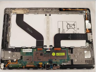
Remove the black back cover with a blue iFixit opening tools by working it around the perimeter of the case.
