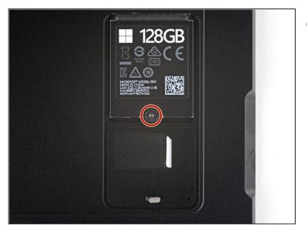
Use a T3 Torx screwdriver to remove the 2.4 mm screw securing the SSD.
