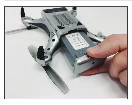
To remove the battery, simply grip the battery by the tabs, press down on both tabs, and pull the battery out.
