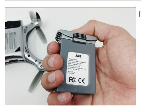
To replace the battery, simply slide it back into its place until the tabs click back into place. If you are having trouble doing this, you may be putting it in upside down. Try flipping it over and trying again.
