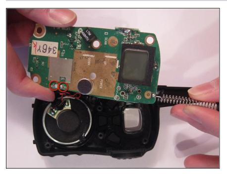
Reattach the speaker wires and antenna to the new circuit board using a soldering iron.
