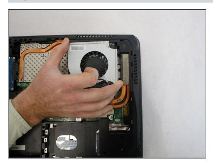
Remove the fan by lifting straight up.
