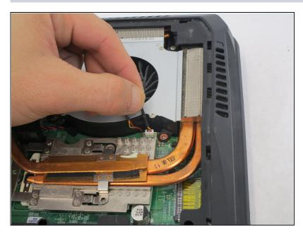
• Disconnect the cable supplying power to the fan.
