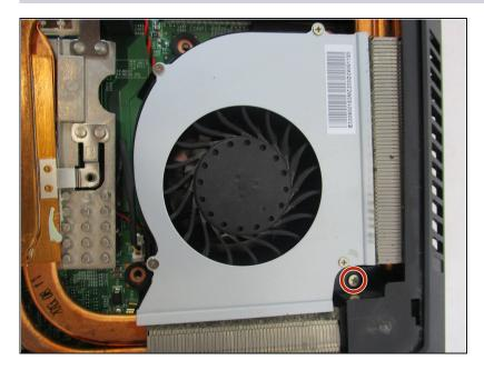
Remove the single 3 mm screw holding the cooling fan in place with a Phillips #0 screwdriver.
