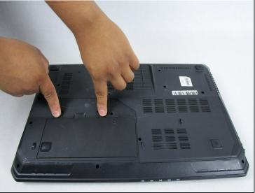
Release the safety latches that hold the battery in place. The left latch will stay moved up, while the right side is spring activated and will have to be held.
