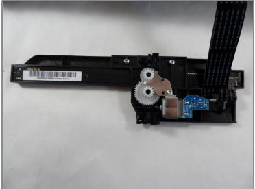
• Remove scanner bar from track inside lid.
