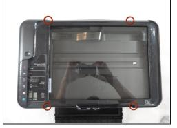
Remove the four 9mm T10 Torx screws on the top.
