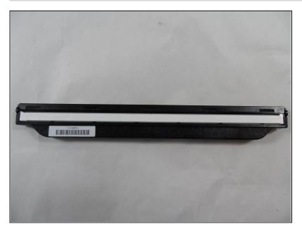
Separate the scanner light from the rest of the scanner bar.
