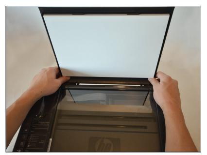
Open the protective lid that is covering the glass. Press gently against the base of the panel to remove the lid from the rest of the printer.
