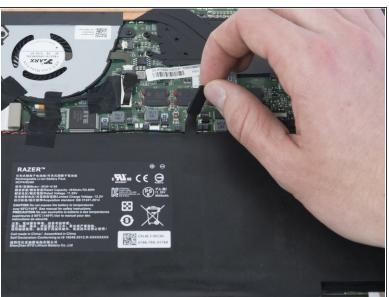
Use your fingernail to pry up and disconnect the battery from the motherboard.
