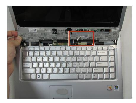
• Carefully lift the control cover up and forward to reveal a single ribbon cable.
