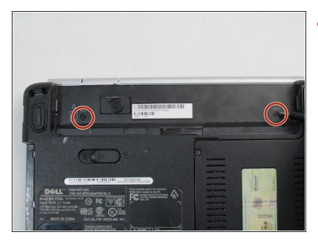
Loosen the two 3.5mm Phillips #1 screws in the battery bay.
