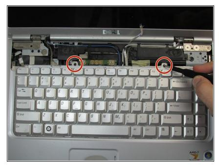
Remove the two 3mm Phillips #1 screws at the top of the keyboard where the control cover was.
