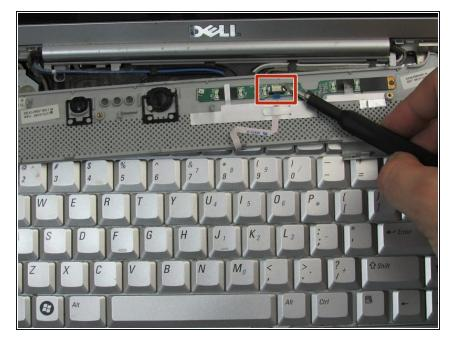
Use tweezers to squeeze the tabs on the connector and remove the ribbon cable.
