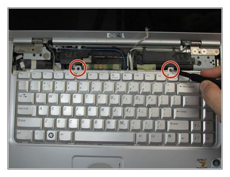
Remove the two 3mm Phillips #1 screws at the top of the keyboard where the control cover was.
