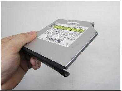
Slide the optical drive out of the side of the laptop.
