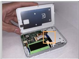
Remove the four screws using the Phillips #00 screwdriver to access the motor and sensor (highlighted in orange).
