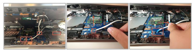
• Using an ESD safe tool, detach all 3 ribbon cables. To do so, lift up the cable up and out.
