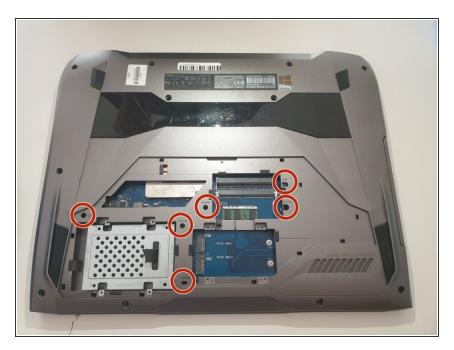
Using the Phillips #00 screwdriver, unscrew the six 5.2 mm screws under the service cover.
