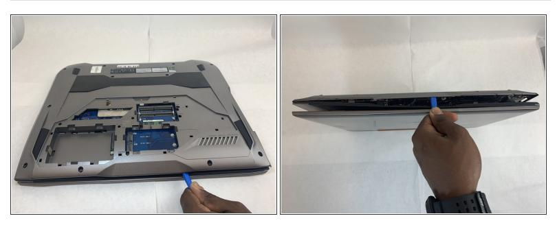
Use the iFixit Opening Tool to pry apart the back panel from the main body of the laptop.
