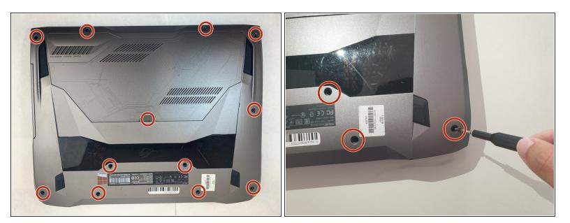
• Using the Phillips #0 screwdriver, unscrew all 12 screws on the back of the laptop.
