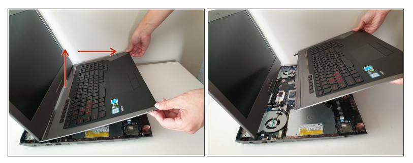
Once the cables are detached, lift the keyboard about 2 inches up and remove it from the rest of the body.
