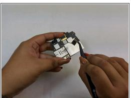
• Using the angled tweezers, disconnect the rear camera from the motherboard.
