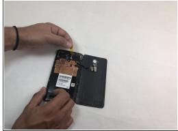
Remove the opaque yellow sticker that indicates where the fingerprint scanner is connected to the back of the device.
