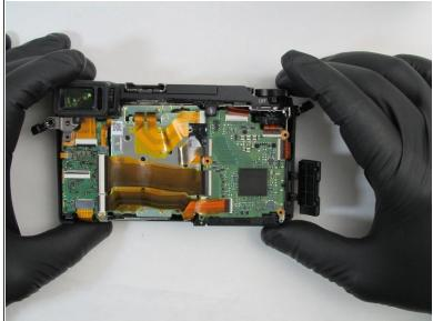
• Remove the three 3.5mm silver Phillips #0 screws mounting the main PCB to the camera frame.
