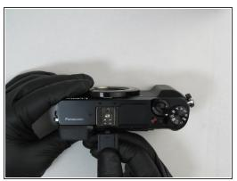
Remove the plastic hot shoe cover by sliding it towards the rear of the camera.
