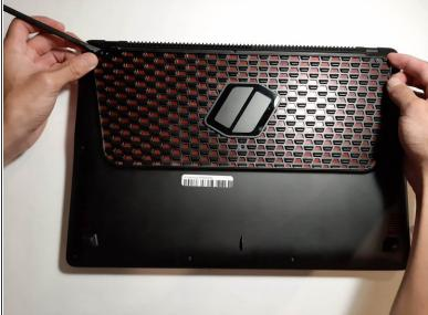
Insert the spudger in one of the top notches of the window and work your way to the other side until you achieve complete separation of the panel.
