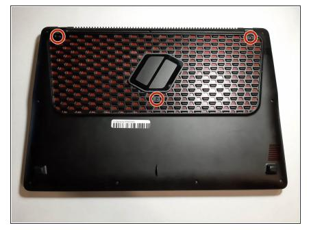
Remove the three 6.6 mm screws on the back of the computer using the Phillips #0 screwdriver.
