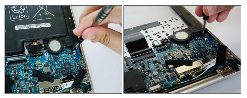
• Remove the screw connecting the speaker component to the motherboard using the screwdriver.
