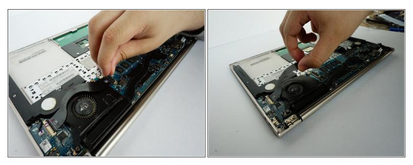
Disconnect the ribbon between the IO and the motherboard on both sides.
