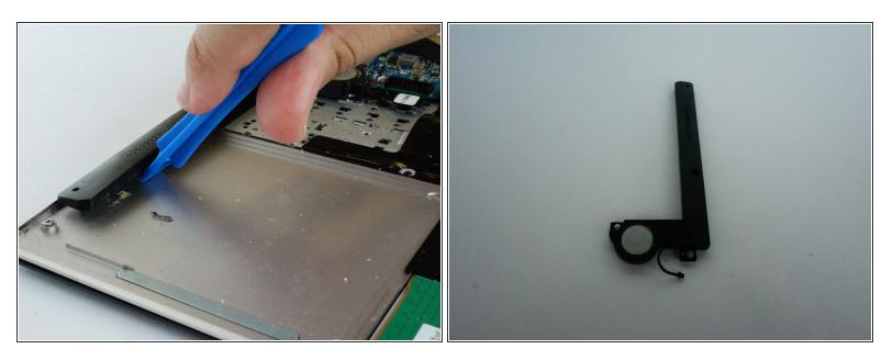
• Using the plastic opening tool, pry open the speaker component from the computer.
