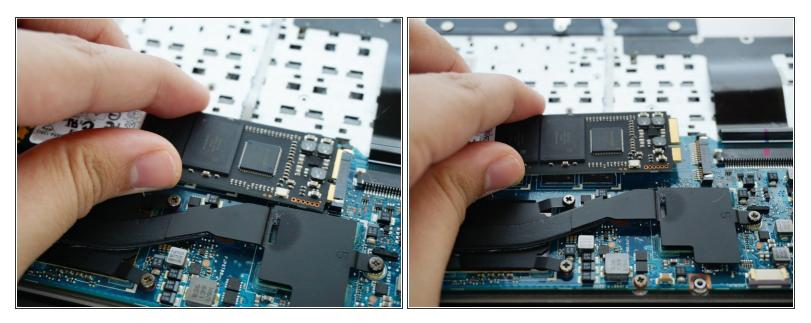
• Using your hand, pull the SSD out from its slot.
