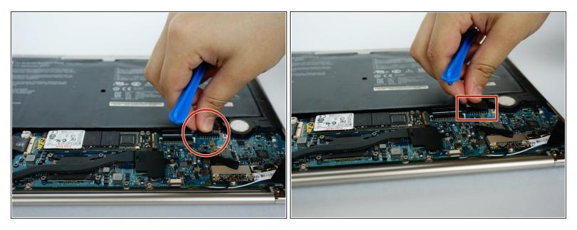
• Disconnect the battery from the motherboard by gently pulling up and down on the connector.
