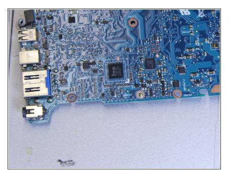
Pull the charging port up from the motherboard with a pair of tweezers while the solder is still liquid.
