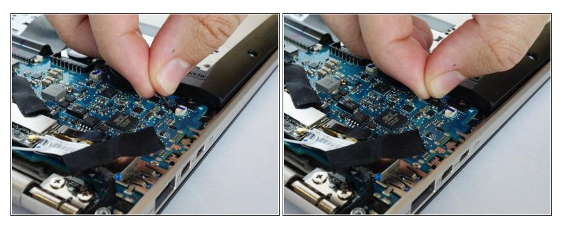
• Disconnect the sound cable from the motherboard.
