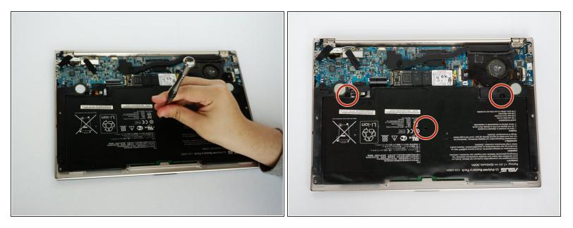
Using the Phillips #00 screwdriver, remove the screws from the middle and the two corners of the battery.
