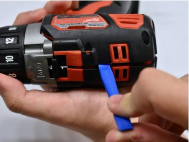
Open the case by sliding the opening tool all the way around the case to pry it apart.
