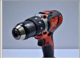
Remove the four 20 mm screws, using the T3 Torx Screwdriver, from the front of the case.
