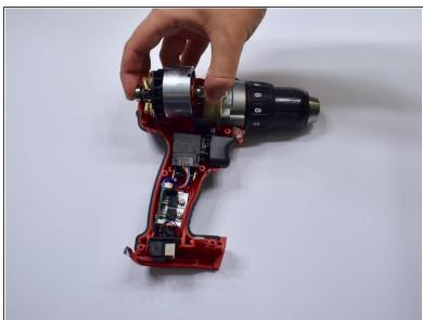
Lift the motor from the casing.
