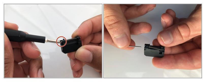
Similar to the previous step, remove the 19mm pin by pushing it from one side using the pointed end of a spudger.
