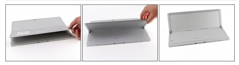
Lift the kickstand about 90° to reveal the hinges.
