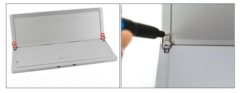
Remove the four 2.7 mm T3 Torx screws, two from each hinge.
