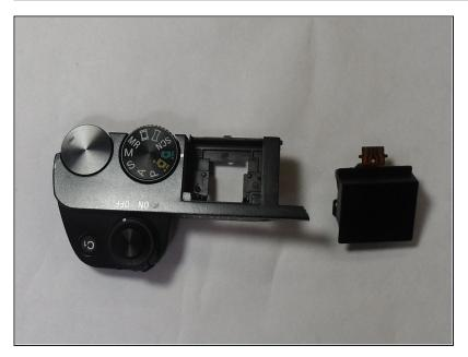
Carefully remove the flash assembly from the top pannel
