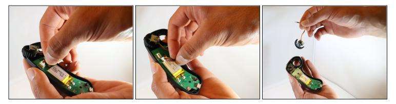
• Unplug the connector and remove the accelerator cable.
