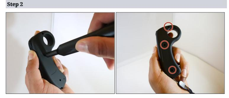
• Using a Phillips #1 screwdriver remove the three screws.
