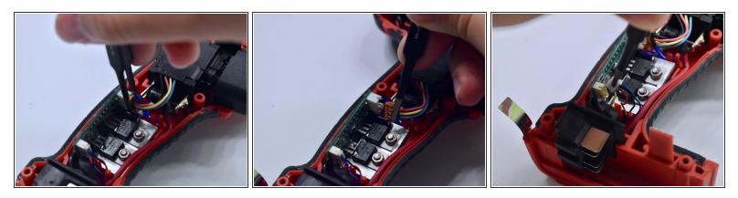
• Remove the 4-pin and 5-pin connector, using the tweezers, from the circuit board.
