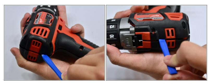
• Open the case by sliding the opening tool all the way around the case to pry it apart.
