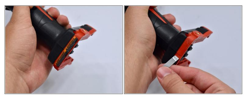
• Peel back the sticker at the bottom of the drill handle.
