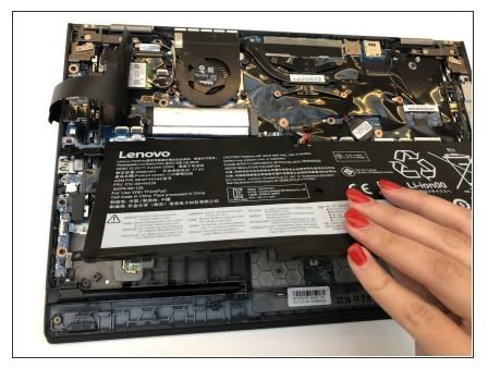
Lift and remove the battery away from the computer. To reassemble your device, follow these instructions in reverse order.
