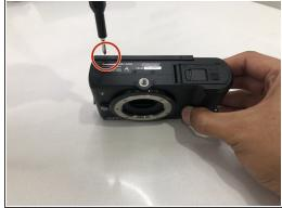
Remove the two 2mm Phillips #0 screws on the bottom of the screen.
