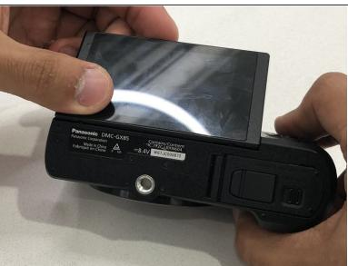
Swivel the screen away from the camera body so it is facing the ground.
