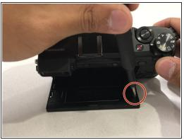
Remove the two 6.0mm Phillips #0 screws on the back of the screen.
