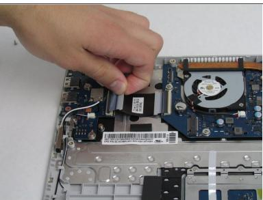
Remove the black ribbon cable by pulling up on the black cover and sliding out the cable.
