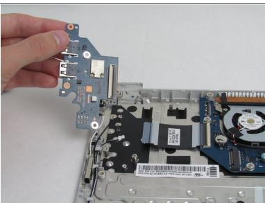
Use the Phillips #00 screwdriver to remove the two 4.5mm screws holding the USB board down and remove the board.
