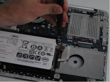
• Use a Phillips #00 screwdriver to remove the three 4.5 mm screws holding the battery in place.
