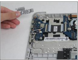
Use the Phillips #00 screwdriver to remove the two 4.5mm screws holding the cover plate in place.
