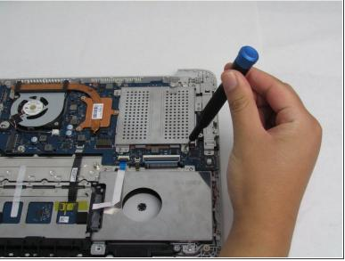
Use the Phillips #00 screwdriver to remove the five 4.5 mm screws.
